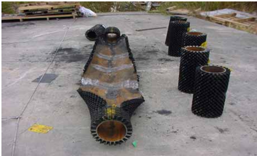
Fig. 8 : Ruptured Tube Detached from the Heater Convection Box
