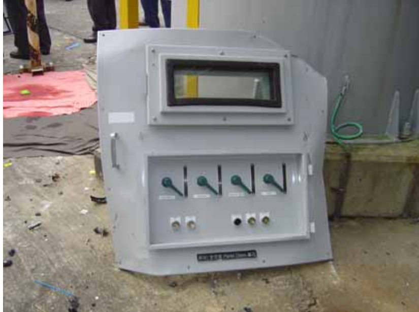
Figure 1: Damaged compressor operating panel cover after explosion(weight about 60kg)
