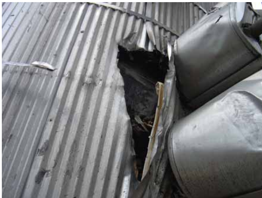
Fig. 3: Impact mark on the adjacent drum by exploded compressor panel cover
