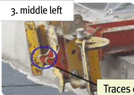
Climbing shoe, which supported the fallen RCS 3
