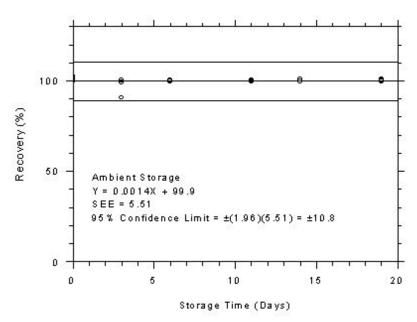
Charcoal tubes ambient storage test, 240-minute samples at 200 ppm.
