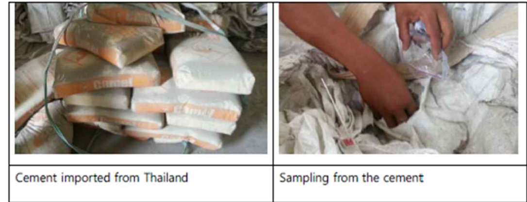
Figure 8 Cement suspected to contain asbestos
