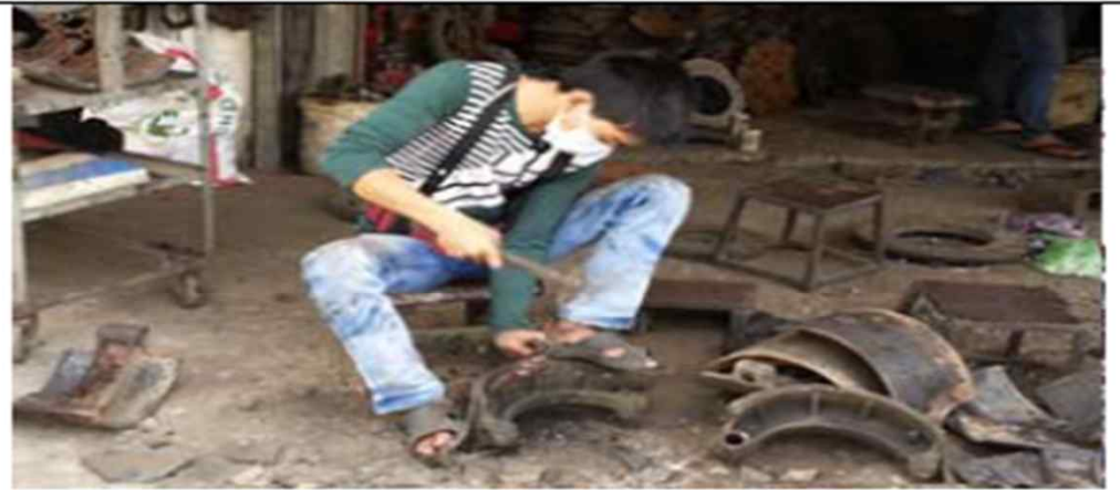
Detaching an used brake pad from a lining
